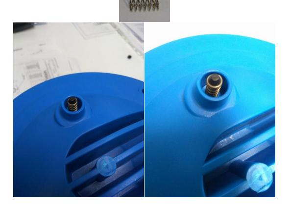
Step 4: Then add the cylinder with the small opening facing up- it will click down over the spring
