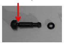
Step 2: Push the small end of the shaft into the vent button hole from the bottom of the filter lid
