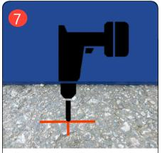
Using a 1/2" masonry drill bit, drill a hole in the concrete. The depth of the hole should be at least 3" deep
