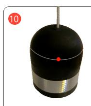
Drill a 1/4" hole through the level indicator through the shoulder/mold line. This line is the correct height for the eyebolt.
