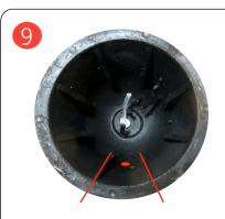
Remove level indicator cap. The level indicator has internal ribs which strengthen the indicator. The hole for the plastic eyebolt should be drilled centrally between these ribs, so that the plastic nut fits between the ribs
