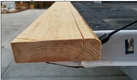
Saw a blades width, 5/8" deep groove cut, 1" from the back of a 2 x 6 lumber board then place on back of truck tail gate or other flat surface.
