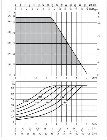
The performance curves are based on kinematic viscosity values =  $1 \text{ mm}^2/\text{s}$  and density equivalent to  $1000 \text{ kg/m}^3$ . Curve tolerance according to ISO 9906.
