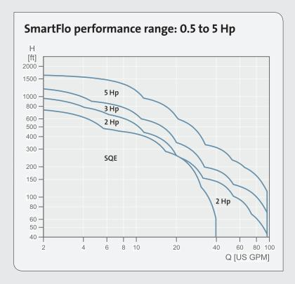
The SmartFlo range comprises systems based around an SQE pump (available in four sizes: 0.5, 0.75, 1, and 1.5 Hp) or an SP pump (2, 3 or 5Hp). The choice of pump size means that you can get constant pressure the SmartFlo way for everything from small single-family homes, to larger homes with extensive irrigation, to small commercial applications. See the performance curve above for details.
