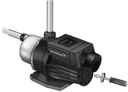
Fig. 17 Removing the end-cover plug
